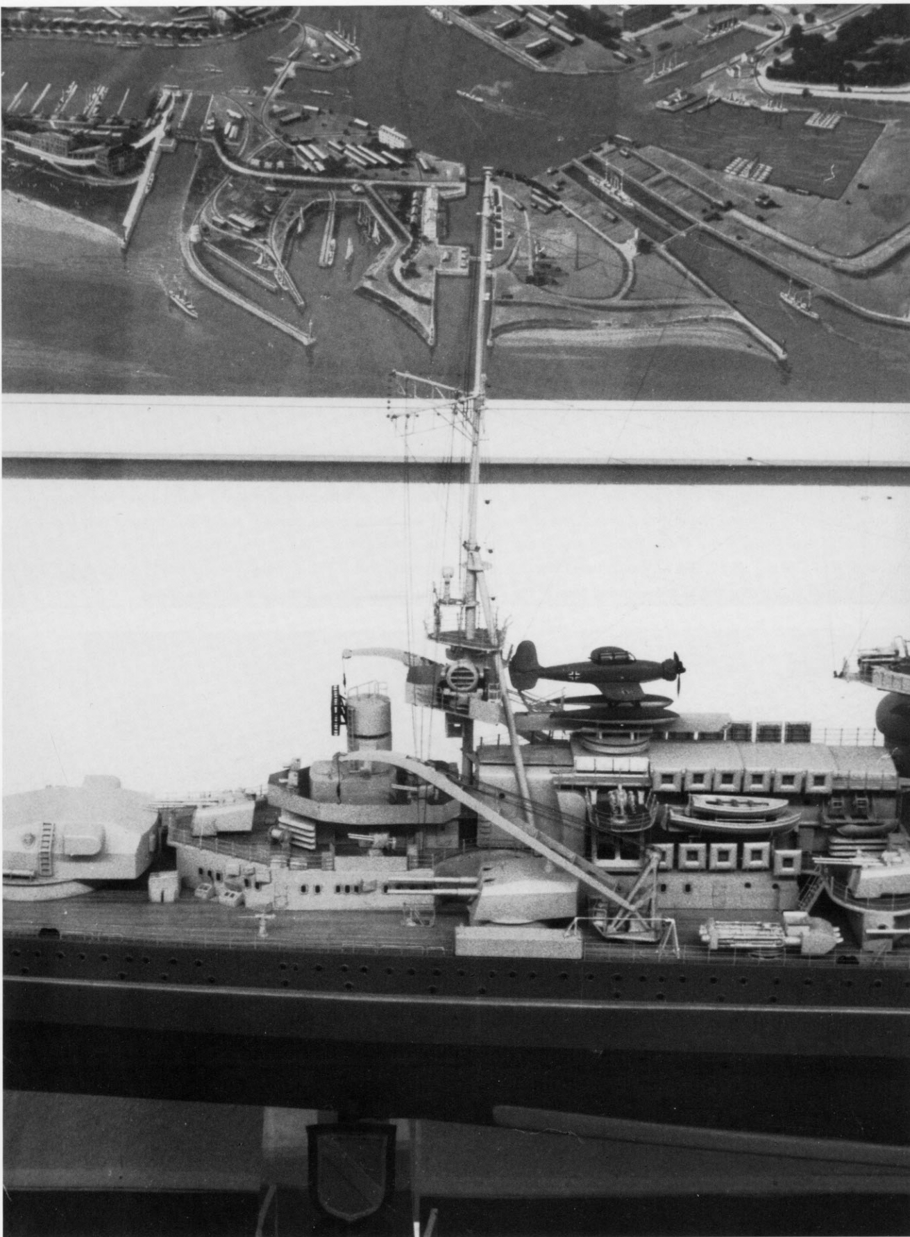
Another sectional view of the midship with the mainmast. Note the many Marx-floats stored on the side of the aircraft hangar. On photographs of the original ship these floats can seldom be seen. Such a float consisted of a square frame, the floating body of which was made of metal or other materials. It was hollow and filled with a water-resistant and floatable material, the inner part fitted with grating. Marx-floats served as additional means of rescue. Under normal conditions they were quite useful but during a battle there was a danger of them being damaged or destroyed by direct hits or splinters, rendering them useless.
