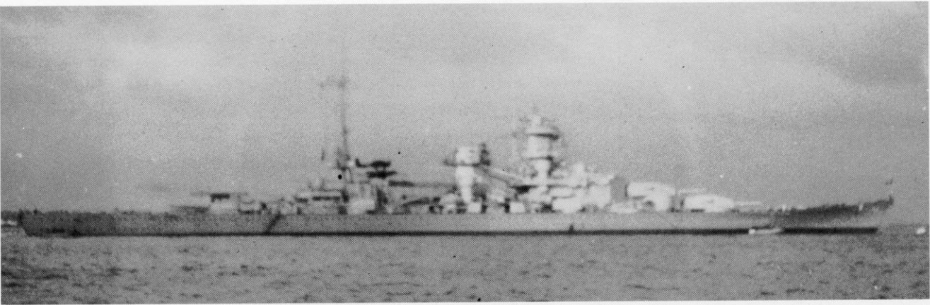
Scharnhorst in the Firth of Kiel after her refit. She is now equipped with an Atlantic bow and a funnel cap; the mainmast was moved further aft, and the hangar was modified. On the front catapult, an Arado Ar 196 can already be seen.
