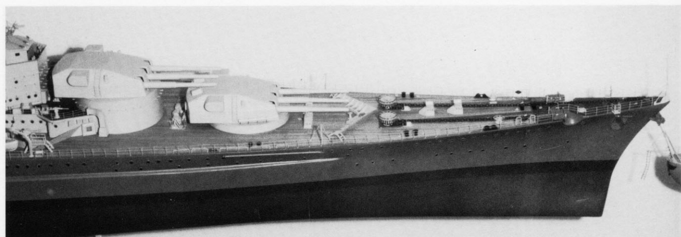
The forecastle with a view of the bow with the front anchor and the swinging boom. The two side anchors lie in their hawses on deck, held by the chain cables coming from the chain lockers and the capstans. In front of 28cm turret A is the breakwater, and there are a large number of scuttles on the ship's side. This model is meant to show Scharnhorst at the time of her leaving Brest but there is one mistake: by this time, 28cm turret A was no longer fitted with a rangefinder and the openings had been sealed with armour plates.
